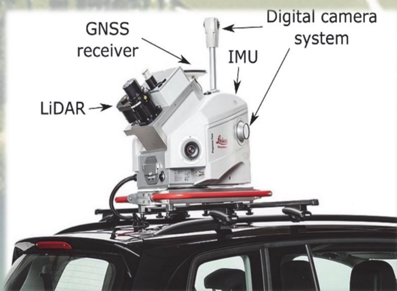
Mobile Mapping System with LiDAR and GNSS Components
